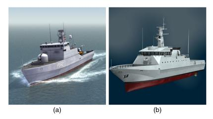
**Fig. 1** Rendered images of the two maritime vessels used: (a) Flyvefisken class patrol boat and (b) offshore patrol vessel OPV54 Pluvier.
